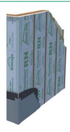
PlastiSpan<sup>®</sup> RN insulation applied to the exterior of above-grade wood frame walls is a great way to increase the energy efficiency of that portion of the home. PlastiSpan RN insulating sheathing is manufactured with the long edges routed out to fit a 19 x 64 mm (1" x 3") nailer. The recessed nailer provides a flat surface for the installation of exterior cladding.
